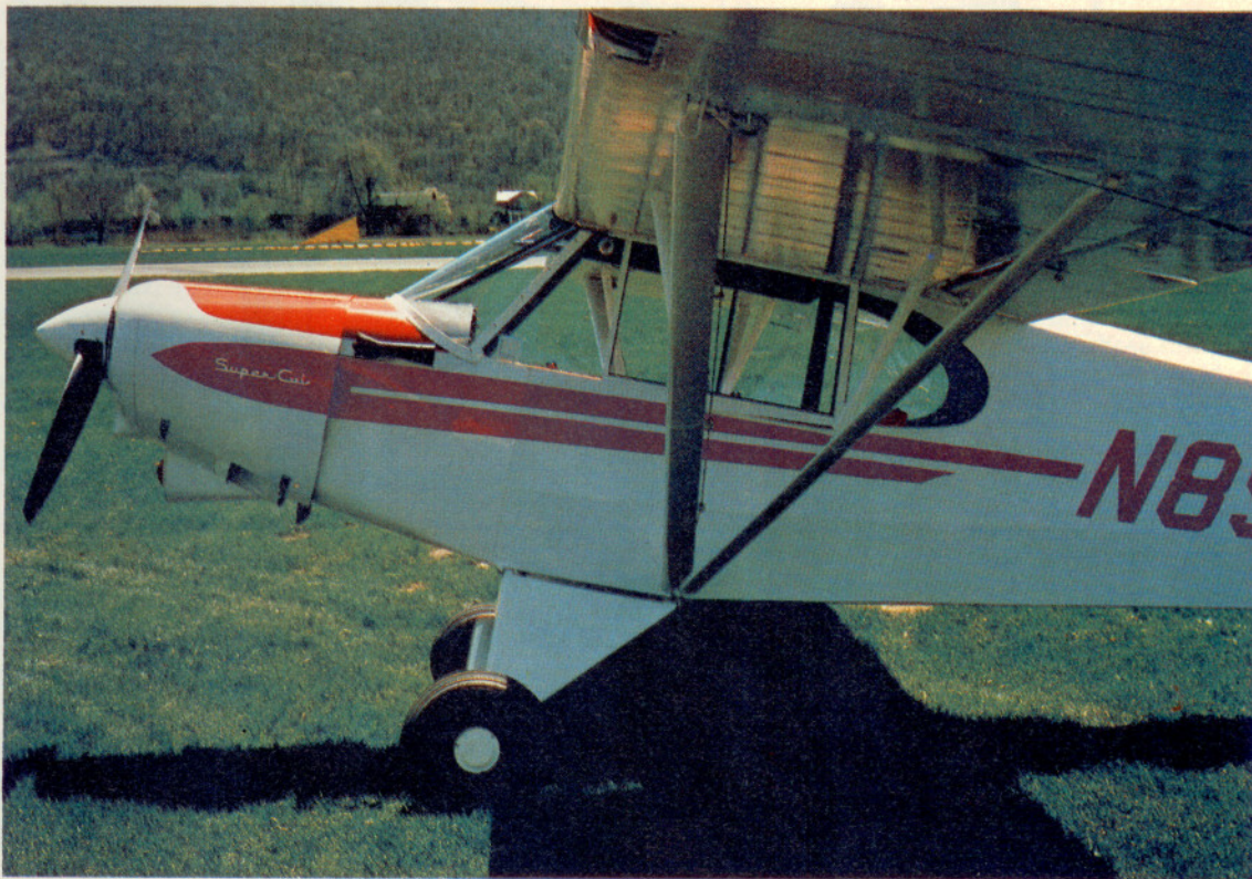
The 150-hp Lycoming up front and the curved metal cowl are Super Cub variations on the J-3 theme.
